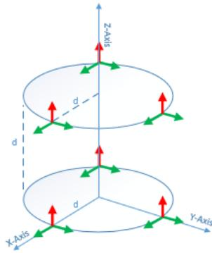
Figure 9. Configuration 6: 18 accelerometers. Arranged in 6 triads around 2 circles with radius  $d$  and a distance  $d$  between them
