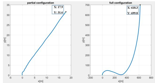
Figure 4. Position error for a constant velocity scenario using the designed GFINS configuration mounted on the ground robot
