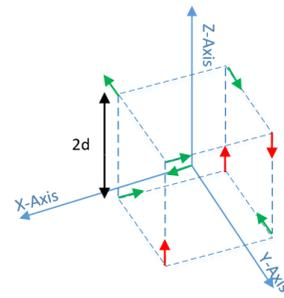
Figure 5. Configuration 2: 9 accelerometers. 1 in the origin and the 8 others arranged on each vertex
