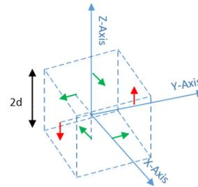
Figure 6. Configuration 3: 6 accelerometers. Arranged on the center of each face
