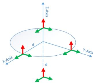
Figure 10. Configuration 7: 12 accelerometers. 9 arranged in 3 triads on a circle within radius  $d$ , another triad in on the  $z$ -axis at distance  $d$  from the origin
