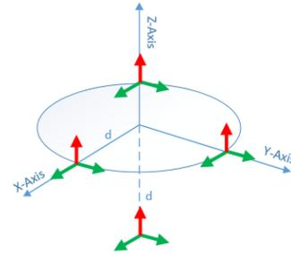
Figure 1. 12 accelerometers configuration. 9 are arranged in triads on a circle within radius  $d$ . Another triad is on the  $z$ -axis at distance  $d$  from the origin. The red arrows are accelerometers which are not used in the partial GFINS
