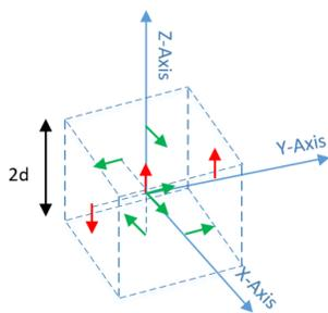
Figure 4. Configuration 1: 9 accelerometers. 3 in the origin and the 6 others arranged on the center of each face
