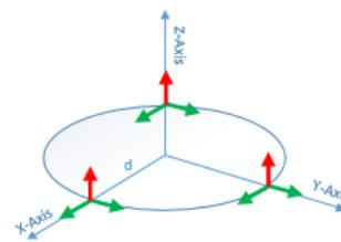
Figure 8. Configuration 5: 9 accelerometers. Arranged in 3 triads around a circle with radius  $d$
