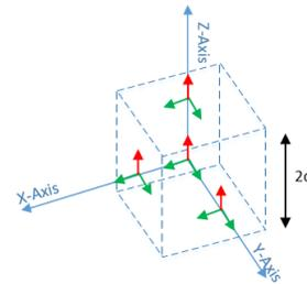
Figure 7. Configuration 4: 12 accelerometers. 1 triad in the origin and the other triads are on the center of 3 orthogonal faces
