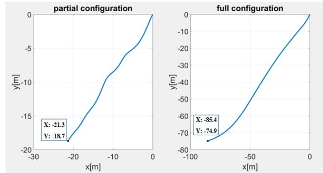
Figure 3. Position error for a stationary scenario using the designed GFINS configuration mounted on the ground robot
